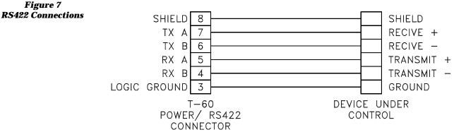
To perform RS485 serial communications with the T-60, the RS422 transmitter and receiver lines must be tied together. Since the RS422 transmitters are disabled after power up, it is safe to assume that no line driver conflicts will occur. Again, refer to the RS422 Statement in the EMERSON EMC BASIC PROGRAMMING GUIDE. The electrical connection between the T-60 and the device under control are shown in Figure 8.
